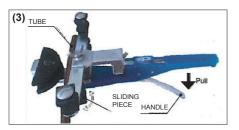
Prepare before bending - placing a tube
