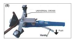
Bending finished - take the bended tube out Upright the bender and pull out the feed lever. univer sal crossbar holder with dented rod retract back will under the effect of gravity. take the bended tube out. if the bended tube get stuck in the former slot, remove them from housing together. (refer to 5 step of tube bending instruction)
