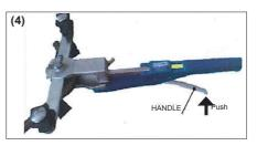
**Bending - push the feed lever repeatedly** Push the feed lever repeatedly until the tube is bended to a certain angle you need. Notice:maximum angle is 90°
