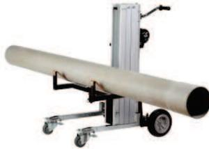
3. Rotating winch handles firmly towards the mast for raising.
